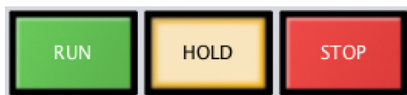
Figure 7.11: The G-code execution control buttons
