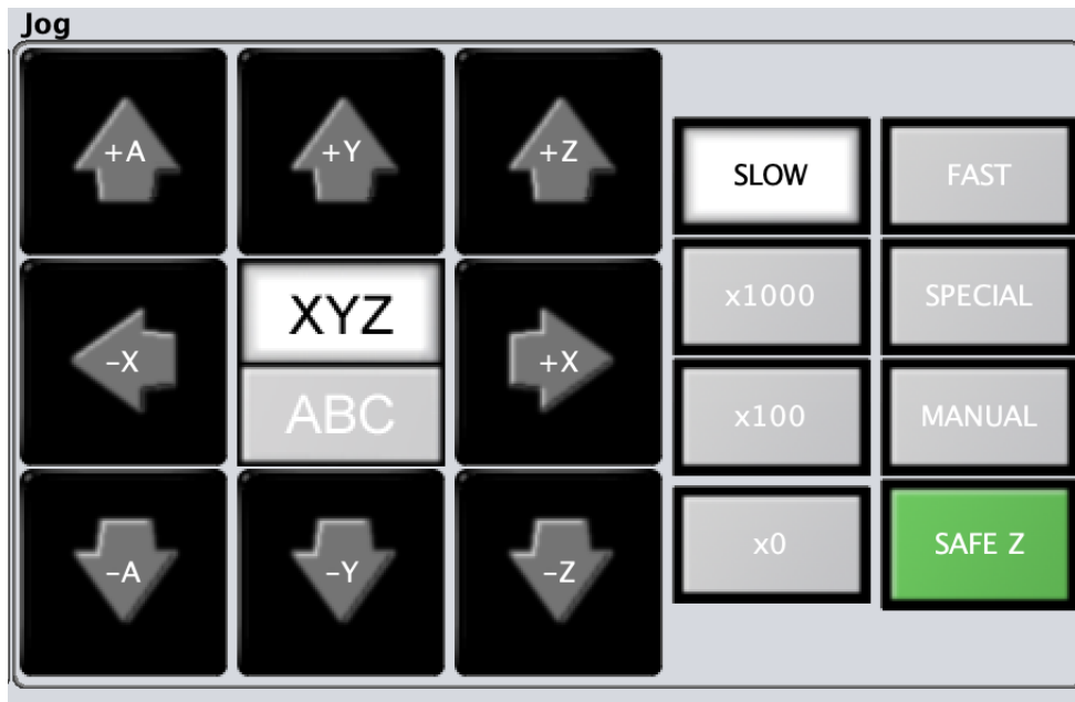
Figure 7.8: The Jog control buttons
