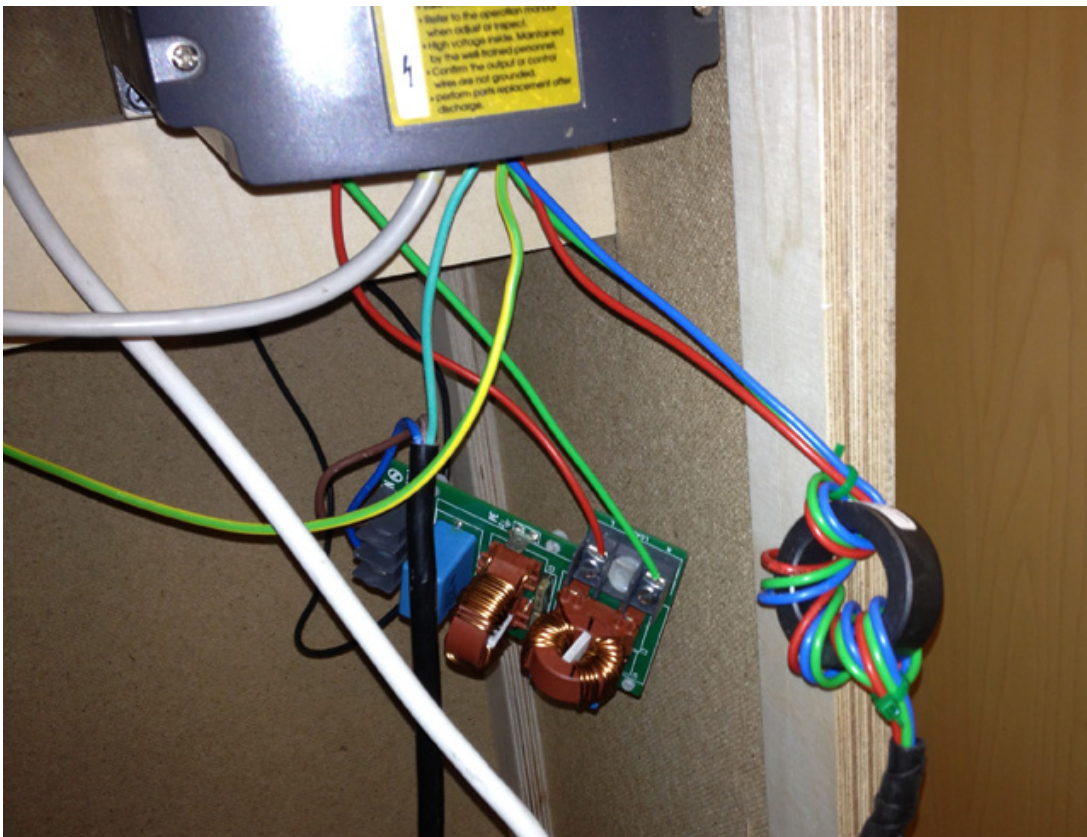
Figure H.1: A picture of EMI filters for a cheap VFD
